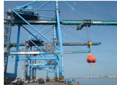
Lomatech testing an 100t dock crane
