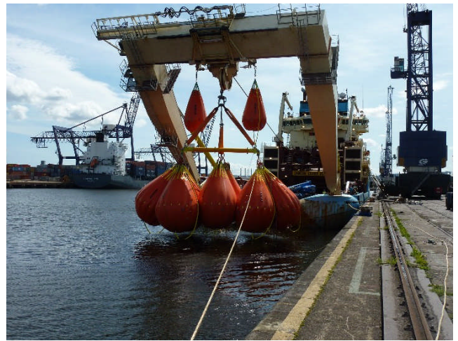
Austin & McLean 300t Load Test on Maersk Advancer
