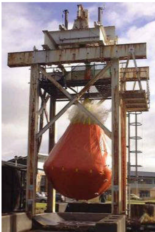
35t WLB being successfully type tested at TUVNEL Ltd. Glasgow.
